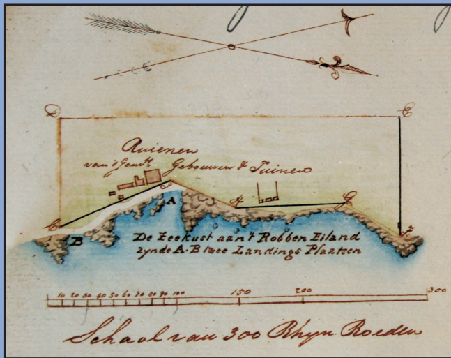
This diagram or map represents the first surveyed portion of land on Robben Island and was placed on the head of the first Deed of Grant to the whaler John Murray. The area was 26,8537 Hectares in extent, and is still reflected as a component of the present day Surveying diagram of the island which can be seen elsewhere in this feature. (Photograph: L J Vosloo)
