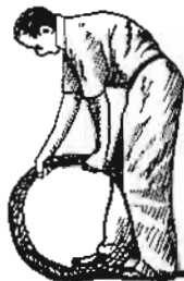
PROPER METHOD OF UNCOILING WIRE ROPE.
