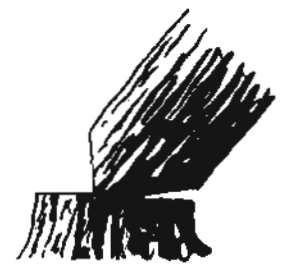
FIG. A.86. THE BRIDGE ACTS AS A HINGE.
