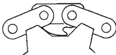
UNDERSIZED SPROCKET BENDS UP TANGS.
