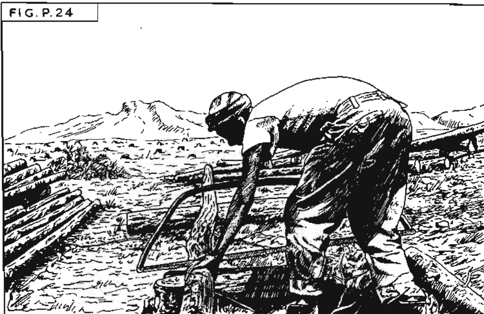
CROSSCUTTING POLES BY ONE-MAN BOW-SAW.
